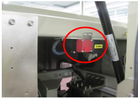
↑ Equipment installed with safety lock device and function maintenance
